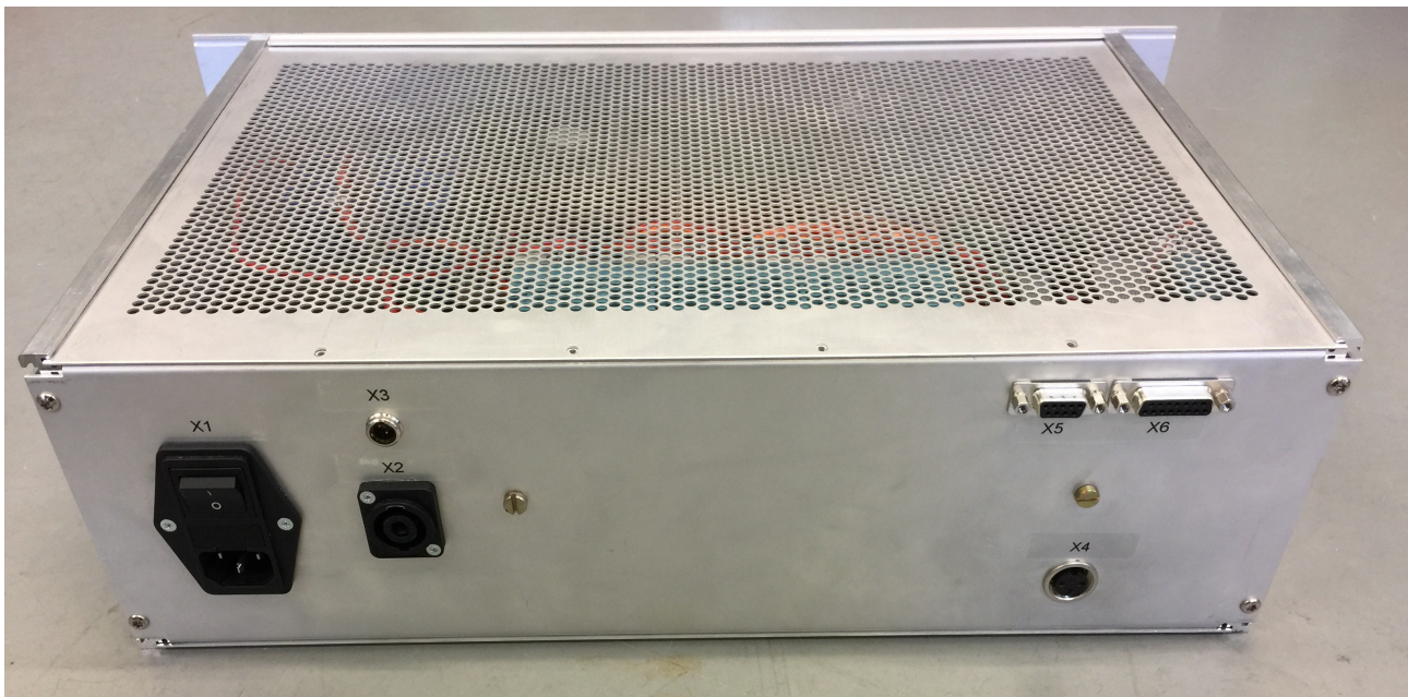
Illustration 1: Overview of the backside of the BX17 generator, including all interfaces
